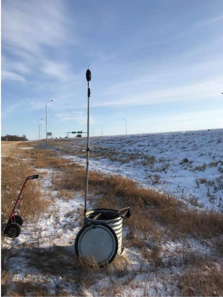
Figure 4.1: Sound Level Meter Including Environmental Enclosure
